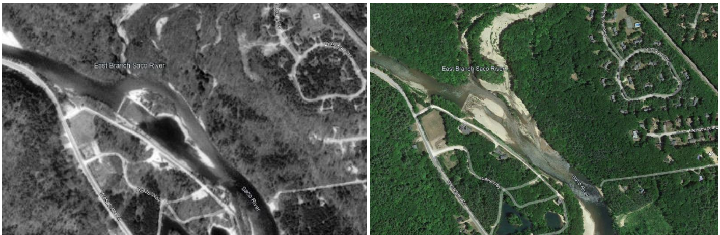
Figure 10. Google Earth Imagery of Kalil Dike in 1994 (left, approximately eight years after installation) and 2018 (right, approximately 30 years after installation). The two time points show how the river geomorphology has shifted and how sediment has accumulated downstream of the dike.
